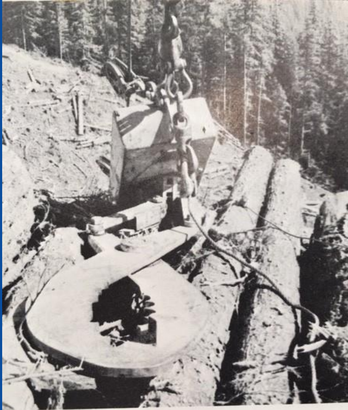
View of "The Snapper" showing simplicity of hook-to butt rigging and grapple swivel detail.
