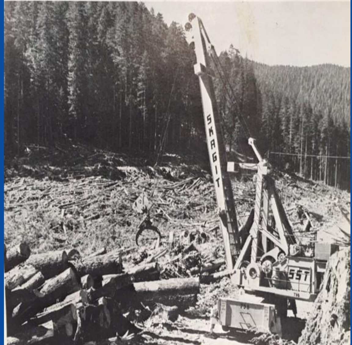
Late model GT-5, Series D, Supertower. Jillpoke has been replaced with two hydraulic guyline drums.
