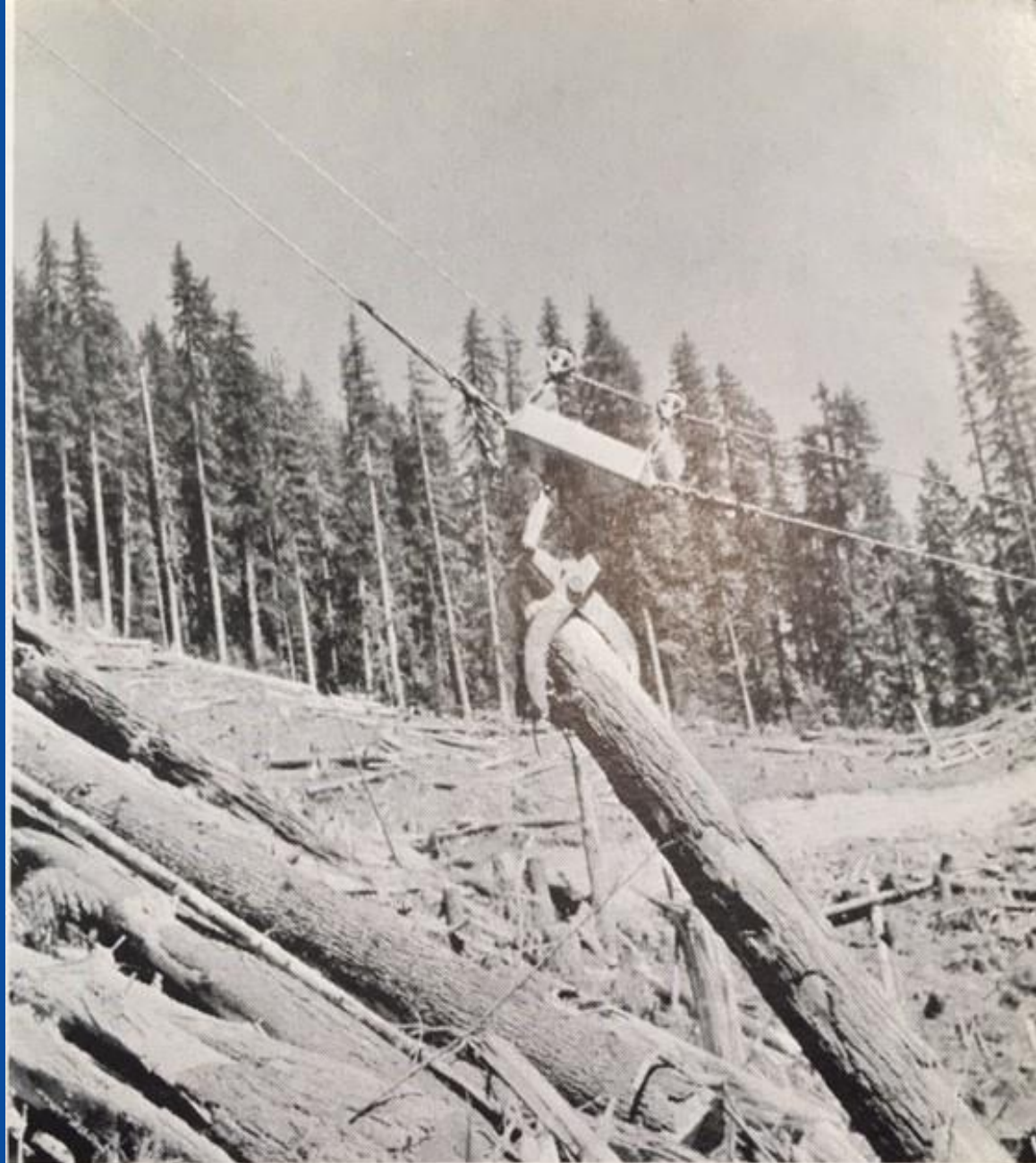
"The Snapper" in operation. Note bell for choker and absence of opening and closing lines.
