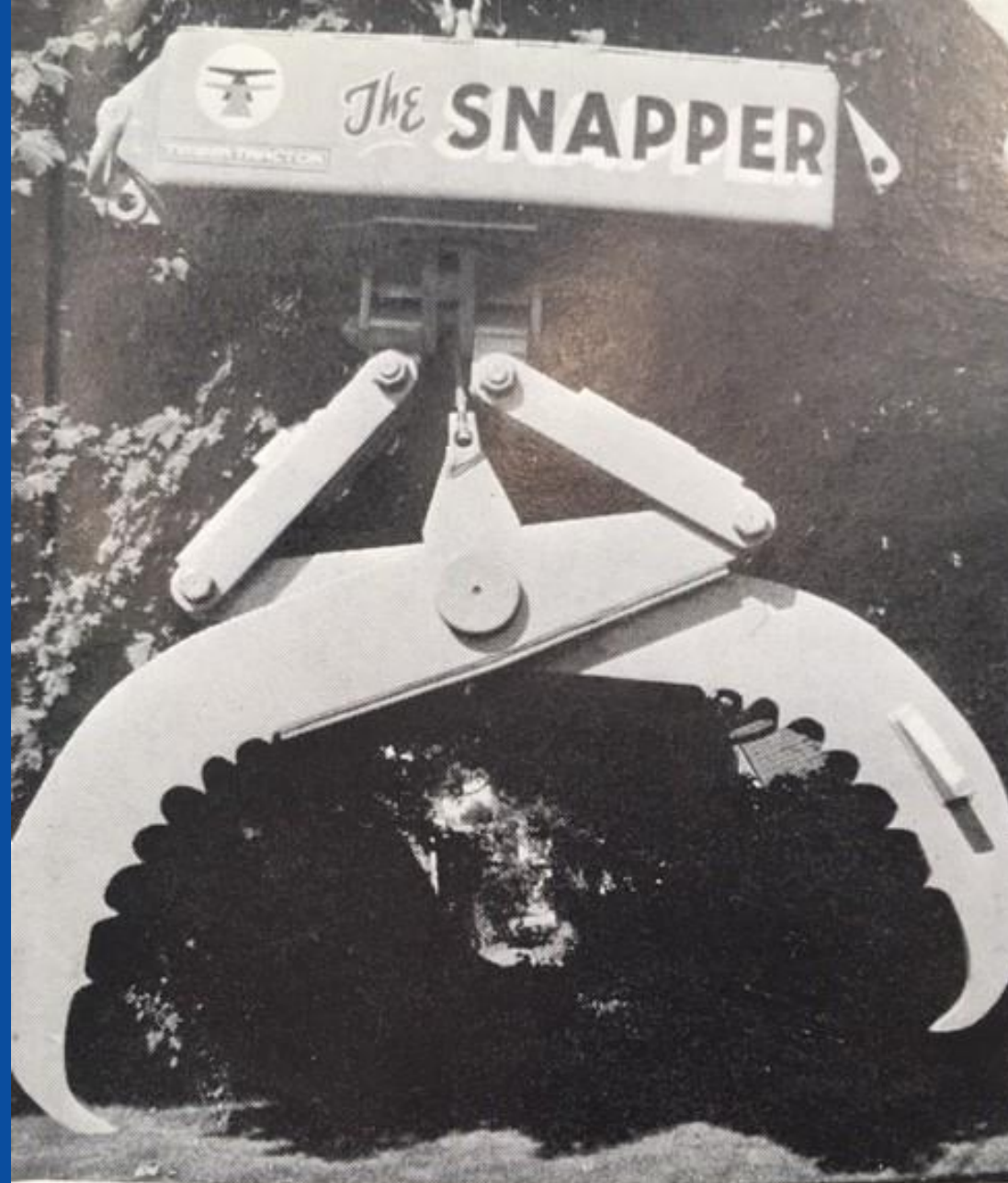
"The Snapper", Battery Powered, Radio Controlled Grapple Carriage.
