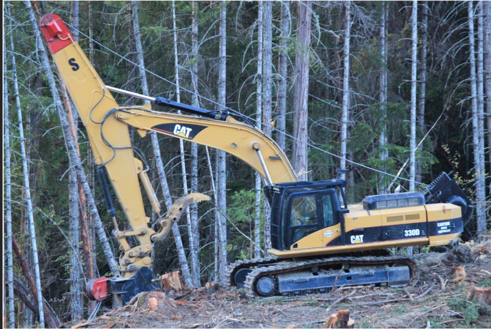
330D Cat Excavator with Summit Machinery winch and tether modification.
