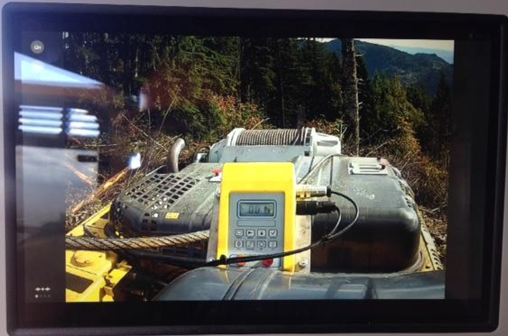
CUTTING MACHINE HAS LIVE VIDEO SHOWING WINCH OPERATION & LOAD CELL READOUT
